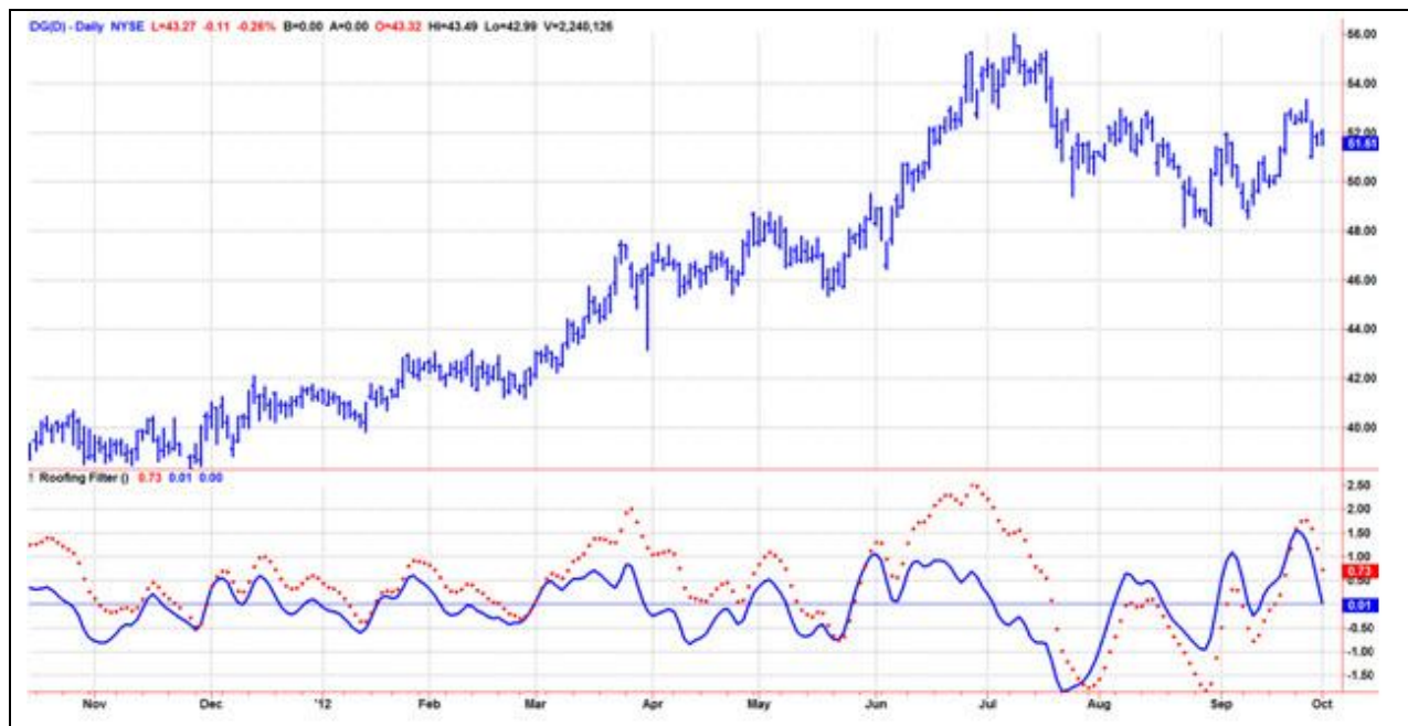
Figure 4. A Two Pole HighPass Filter Removes the Effects of Spectral Dilation. This Gives the Oscillator a Zero Mean to Accurately Asses Turning Points and Generally Reduces Indicator Lag.
