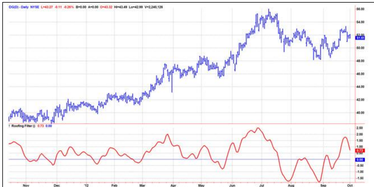
Figure 3. A Single Pole HighPass Filter (or Oscillator) Does Not Remove Low Frequency Components, Resulting in the Output Failing to Have a Zero Mean
